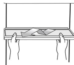
2. Remove the Vegetable & Fruit Drawer by pressing on the indentations found on the inside left and right sides of the Veggie Box/Dry Box cover and remove by pulling forward. Holding the drawer with one hand, lift it up a little bit while pulling it forward and take it out of the refrigerator.
