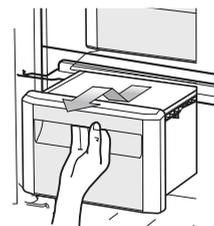
4. Remove the Ice Box from the shelf, then lifting the shelf up and pulling it out from freezer.
