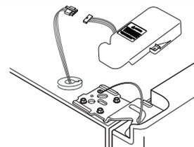
3. Place the front part of the upper hinge cover **9** on the front of the upper hinge **10** and reattach with the screw.
