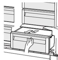
3. Remove the Gallon Door Bin by holding the bin with both hands and gently lifting it up.
