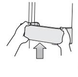
4. Push the Case Fixer handle, and lift the Water Tank up, then take it out
