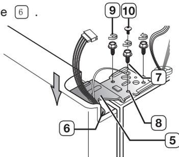
3. Reconnect the wires and place the front part of the upper hinge cover **11** on the front of the upper hinge **12** and reattach it with the screw.
