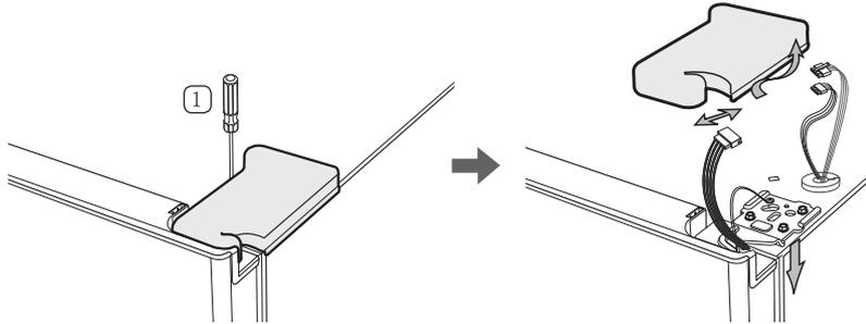
2. Remove hinge screws **2** and the ground screw **3** by turning counter-clockwise, and take off the upper hinge **4**. Be careful that the door does not fall on you as you are removing it.
