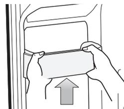
3. Remove the Plastic Drawer by pulling it out and slightly lifting it up.
