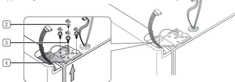
3. Remove the door from the lower hinge **5** by lifting the door straight up **6**.
