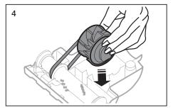
• If the belt is broken or cracked, replace it with a new belt following the instructions above.
