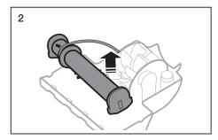
• If a clog is present or debris is visible, inspect the brush roll.
