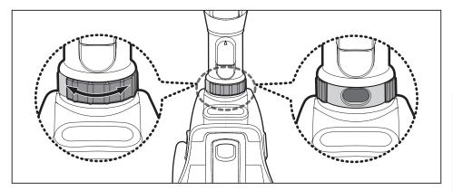
Due to the suction power of this vacuum, it may become necessary at time to adjust the suction power on the handle. If the vacuum seems difficult to push or pull on high pile carpets and area rugs, adjust the suction power by rotating air tap 180° to open valve. Rotate the air tap to close the valve when you need high suction and for vacuuming floors.
