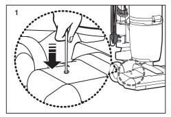
The overload protector shuts off the brush motor if the Motorized brush becomes obstructed. To reset the overload protector, use a pen tip to press the reset switch.
