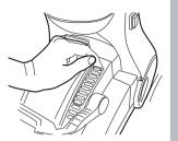
Remove the exaust filter chamber.
