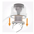
Pull to remove the shroud out of the dirt container.
