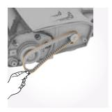
Remove the belt and clean any belt residue from the spindles before replacing the new belt
