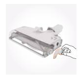
Lift and remove the top part of the brushbar side cover.
