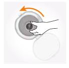
Line up the tabs on the separator into the dirt container. Twist the separator anti-clockwise to lock into place.
