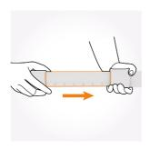
Slide the adjuster on the telescopic extension tube and select required length.
