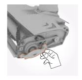
Pull and remove the brush bar location plate.
