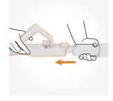
Line up hose handle with telescopic tube. Push hose handle into telescopic tube until clicks and locks into place.
