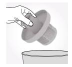
Tap the shroud over a bin to remove any dirt/debris. Using a soft brush remove any remaining dirt/debris from the shroud.
