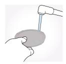
Tap the pre-motor filter over a bin to remove any dirt/ debris. Wash the filter under running water (40°C max).
