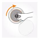
Twist the shroud clockwise to unlock.
