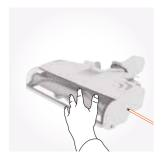
Using a crosshead screwdriver, remove 3 screws from the side of the floorhead and remove end cap belt cover.
