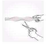
Using scissors remove any threads or hair from around the brush bar and clear any dirt or debris from powered head.
