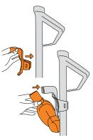
Push TurboTool holder on to the handle and clip TurboTool into position
