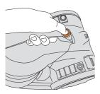
Press dirt container release button to remove the dirt container.
