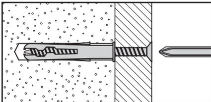
Generally aerated blocks should not be used to support heavy loads, use a specialist fitting in this case. For light loads, general purpose wall plugs can be used.
