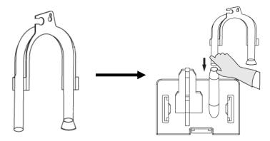
3. The other end of the drain hose can be directly connected to the wastewater drain or to the washbasin. The fitting must always be secured in all types of connections. Your house may be flooded if the hose gets out of its housing during water discharge.
