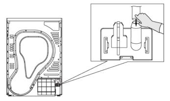
2. Connect the drain hose supplied with the machine to the pipe fitting.
