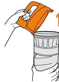
Lift lid to access inner cyclones.
