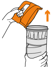
Lift lid to access filter.
