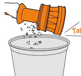
Hold cyclones/separator over bin and tap to remove dirt and debris.
