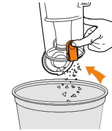
Hold dirt container over a bin and press dirt release button to open, allowing dirt to fall out.
