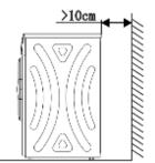
The tumble dryer will expel moist air, and it's recommended this is directed outside to avoid condensation accumulating inside a room. Position the vent hose supplied, through a window or an air outlet so that the moisture can escape. Contact a qualified tradesman to fit the vent hose so it exits through a wall or door.
