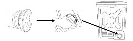
The air outlet hose must be extended directly to the outdoors.
