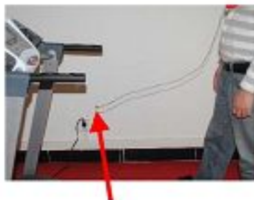
Safety key pin fall off
