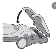
**Refit brush assembly** • Hold the brush assembly and stretch the belt until brush mountings slot down into the cleaner housing. Rotate the
