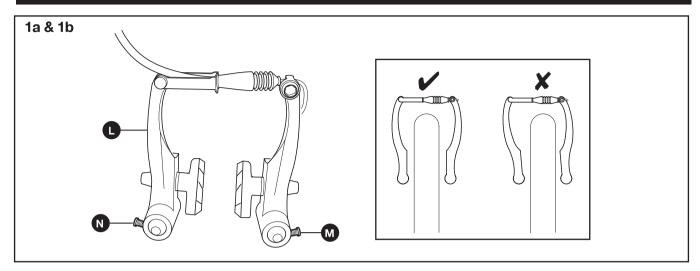
Over time, the brake arms can begin to lean to one side or another making the distance between the brake pads and the wheel rim uneven. This can be corrected by adjusting the spring tension of the individual brake arm.
