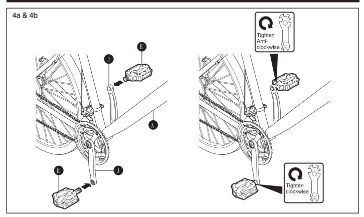
**NOTE!** The pedals **(b**) and crank arms **(J**) have colour coded stickers to indicate which pedal **(b**) matches which crank arm (**J**).
