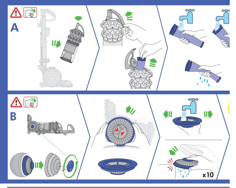
Base plate disassembly
