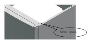
3. Remove middle hinge, screws, screw caps and plastic inserting nails. Install them on the other side. Take off the lower door and put it away.
