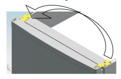
9. Install the top bar cover and a top cover buckle. Screw down the four screws and cover them with caps. Finally insert the top endcap coverslip
