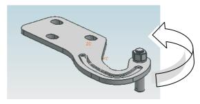
B. Install the assembled top hinge. Screw it down and fix it on target side
