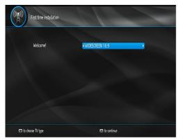
By pressing the "**I**/**>**" buttons select the Tv type you want to set and press OK button. Afterwards, "Select HDMI resolution" OSD will appear on the screen.Select your desired resolution by pressing "**I**/**>**" button and press OK.
