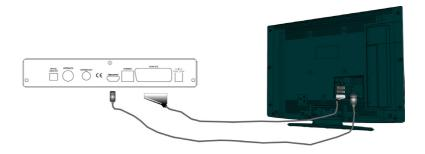
You can connect the set top box to your TV by using the scart socket or HDMI input. Use a scart or HDMI cable to connect the set top box to your TV.
