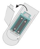
• Remove the battery cover located on the back of the remote control by gently pulling backwards from the indicated part.
