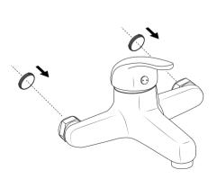
Remove the backnuts and washers from the bath pillars.
