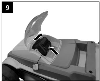
**NOTE!** The battery is stored under the safety flap during delivery. Take out the battery before fitting it (Fig. 8).
