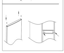
Install the bottom hinge to the left side of cabinet, then install two adjustable feet on the current position, then install the freezer door.
