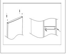
6. Install the bottom hinge to the left side of cabinet, then install two adjustable feet on the current position, then install the freezer door.
