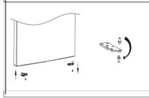
Remove the freezer right hinge hole cover, install to lest side. Remove the center hinge screw hole plug on the left side, then install its to right side.
