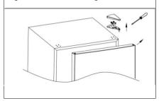
2. Remove two screws that secure the center hinge.
