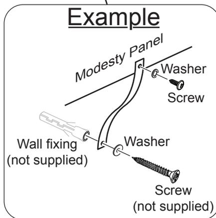
To prevent possible overbalancing this unit must be secured to a suitable wall by fitting of the overbalance protector kit to the unit.
