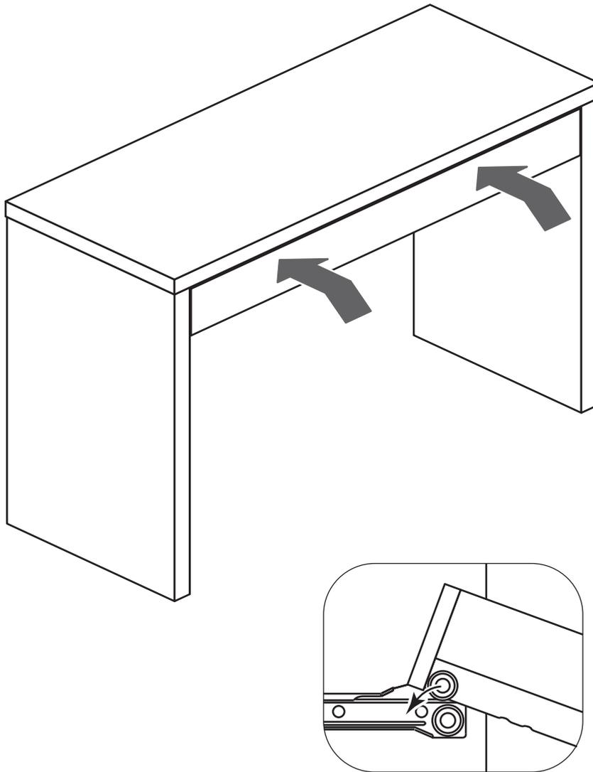
Slide the wheels of the 4 Runners fitted to the Drawer, over the wheels of the Runners fitted to the panels and push the drawer into position.
