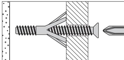
For use with plasterboard partitions or hollow wooden doors.
