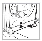
1. Take off the cover panel on the front of the machine by first pressing it in the centre and then pushing downwards on both sides until you can remove it (see figures).
