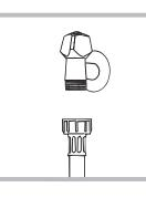
1. Connect the supply pipe by screwing it to a cold water tap using a <sup>3</sup>/<sub>4</sub> gas threaded connection (see *figure*).
