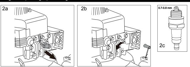
2a Once the engine has cooled, pull off the spark plug boot with a twist. Remove the spark plug using the socket spanner supplied.
