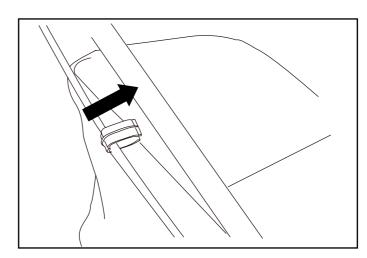
4. Ensure that the cable clips supplied are used to fix the cable to the Lower Handle.
