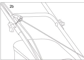
Lift the upper handle, and lock in place using the quick release lever and tensioning bolts that are attached to the handle.
