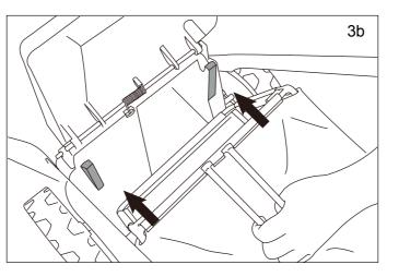
3a. Firstly attach the grass bag to the frame by fixing all plastic hooks.
