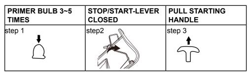
To start the engine, make sure that the spark plug cap is located on the plug and the machine is filled with sufficient oil and petrol.
