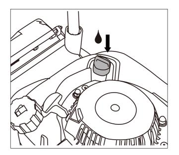
Always use high quality detergent oil classified SAE30 oil (or equivalent eg 5W 30, often termed as 4 Stroke lawn mower oil). Only use additives recommended by the engine manufacturer. To prolong the life of your engine it is important that the oil is changed after the first 5 hours of use. Using non-detergent oil can shorten the engine's service life and using 2-stroke oil will damage the engine.
