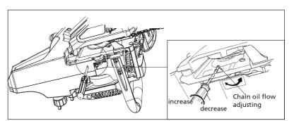
After starting the engine, run the chain at medium speed and see if chain oil is being dispensed as shown.
