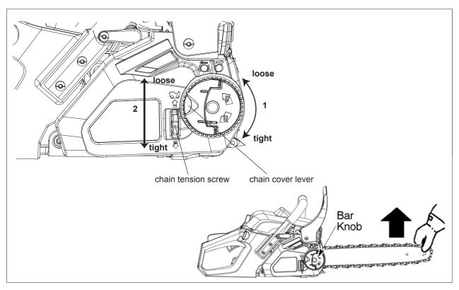
1a Pull the chain cover lever out, and slightly loosen the chain cover.
