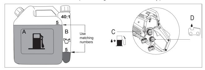
FUEL MIXTURE: 1 Litre (1000 ml) petrol: 25cc (25 ml) 2 Stroke engine oil (40:1 ratio)
