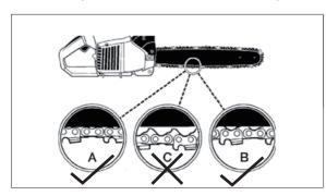
CAUTION! If the saw chain is TOO LOOSE or TOO TIGHT the V-drive wheel, chain bar, chain and crank shaft bearing will suffer premature wear. Above fig. shows the correct tension A (when cold) and tension B (when warm). FIG C shows a chain that is too loose.
