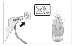
Output the iron and let the soleplate (7) cool down. Wipe the soleplate with a damp cotton cloth only.
