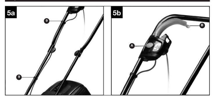
Before you connect the mower to the mains supply make sure that the data on the rating plate is identical to the mains data. Connect the plug to an extension cable if necessary. It is imperative to secure the extension cable to the handle with the cable grip as shown in Figure 5a.
