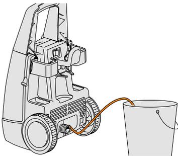
After use rinse the pressure washer to prevent blockages. Inset the solution tube into a bucket of fresh water (Max 40°C), turn the machine on and squeeze the trigger for 1 minute.
