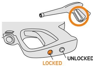
A trigger safety lock is located underneath the handle. The safety lock should always be in LOCKED position before connecting/disconnecting the pressure hose to the trigger handle.
