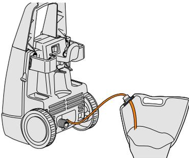
Unhook the solution tube and insert into the solution bag. Solution only dispensed with the trigger handle, lance and solution nozzle, or car/outdoor/rotary brush if supplied.
