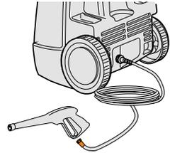
To connect pressure hose to trigger handle, press the pressure hose release button and push pressure hose to lock into position. Gently pull the pressure hose to check the connection.
