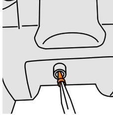
To remove water filter, pinch the inner water filter tab with pliers and gently pull.
