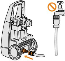
Make sure water supply is not connected. Firmly push the water hose pipe with suitable connector onto the water inlet to lock into position.
