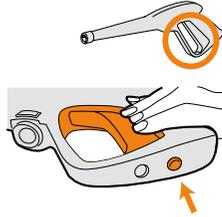
Before plugging the machine in, press the unlock safety button on the trigger handle and squeeze the trigger until water starts to flow through the nozzle.
