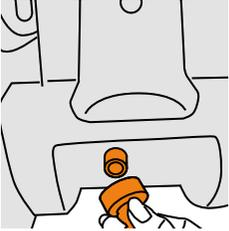
To access water filter unscrew water inlet connector and remove.
