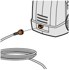
Push the pressure hose firmly to the water outlet and turn the pressure hose collar clockwise until tight.
