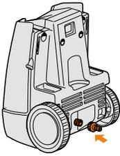
Attach the hose connector to water inlet by turning clockwise until tight.
