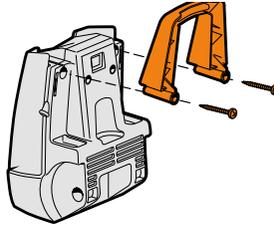
Slot the handle in to the top of the machine and insert the 2 screws, turn clockwise to tighten.
