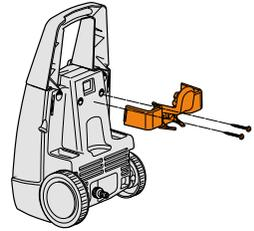
Align the pressure hose and cord storage hook onto the back of the machine and secure with 2 screws.
