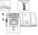
To open the detergent dispenser use the opening device A. Introduce the detergent into the dry dispenser B only. Place the amount of detergent for pre-washing directly inside the tub.
