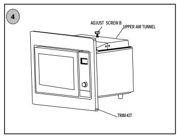
4. Fix SCREW B on the UPPER AIR TUNNEL of the oven.
