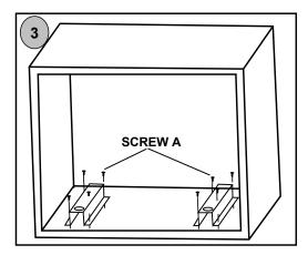
3. Remove the BOTTOM CABINET TEMPLATE, and fix the BOTTOM BRACKETS with SCREW A.
