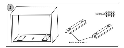
2. Make marks on the bottom plane of cabinet according to marks "a" of the template.
