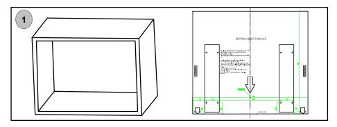
1. Read the instruction on the BOTTOM CABINET TEMPLATE, put the template on the bottom plane of cabinet.
