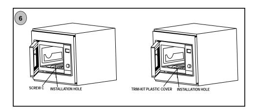
6. Open the door; fix the oven to the cabinet with SCREW C at the INSTALLATION HOLE of TRIM KIT. Then fix the TRIM-KIT PLASTIC COVER to the INSTALLATION HOLE.
