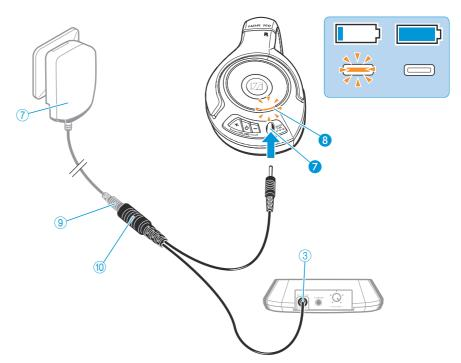
The transmitter automatically switches from battery operation to mains operation if you connect the power supply unit or the charging cable (1) to the transmitter.
