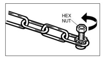
• **To fix the security chains to their anchor brackets:** Loosen the hex nut at the unattached end of the safety chain, until it is flush with the screw end. **Do not remove it completely**.
