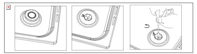
• Unscrew the injector and replace it with the required injector for the new gas supply according to the table below.
