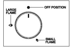
Use the control knob of the relevant burner to set the temperature intensity.
