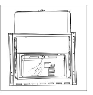
• Unscrew the injector and replace it with the required injector for the new gas supply according to the table below.
