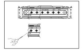
Locate the adjusting screws for the grill and oven burners. These will be positioned to the left hand side of the grill and oven thermostat taps.
