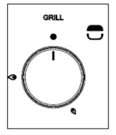
• To turn the grill on press and turn the control dial to the large flame position.
