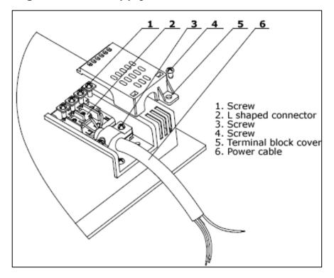
The mains terminal block is located on the underside of the hob and the terminals are accessible by removing the terminal block cover by removing the cover screw.
