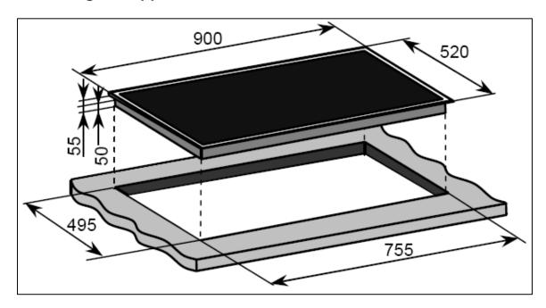
o Cut a hole in the worktop that corresponds with the drawing shown above.
