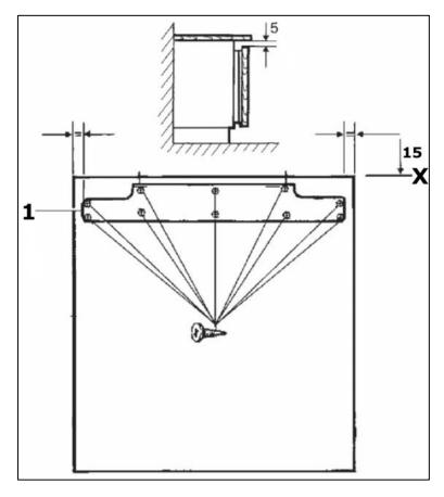
b) Measure the width of the furniture door, at the halfway point mark a line vertically down the inner surface of the furniture door. You should draw the line from the top of the furniture door to approximately halfway down.
