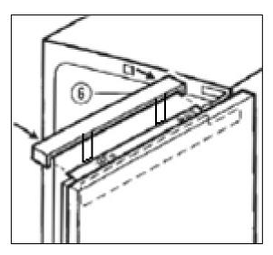
e) Insert the cover plate to the top of the appliance; this will just clip into place.
