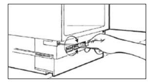
o Remove the grid on the base of the appliance by unscrewing the screws on each side of the grid and then pull the grid towards you.
