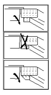
IMPORTANT: There are ventilation holes around the outside of the hob. YOU MUST ensure that these holes are not blocked by the work top, when you put the hob into position (see drawing opposite).
