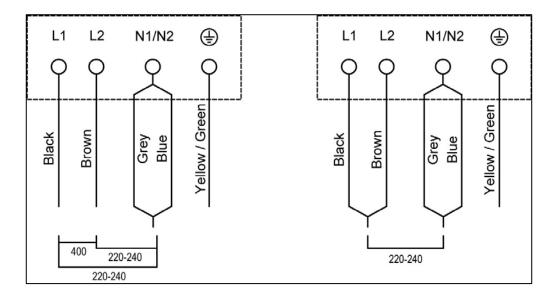
The brass links must be positioned as marked in the appropriate diagram and once established ALL terminal screws must be tightened down firmly.
