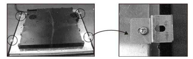
You should place the bracket on the underneath of the hob, in a position that is appropriate for the aperture that you have cut out. Using the screws provided, fix the bracket to the hob. These screws MUST be securely tightened.
