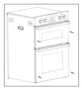
• Ensure that the oven has been securely fixed into the housing unit. The fixing of the oven into the housing is made by using four screws. These should be screwed through the oven cabinet and into the housing unit.
