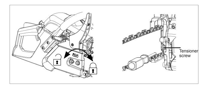
1a Slightly loosen the chain cover nuts.
