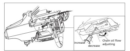
After starting the engine, run the chain at medium speed and see if chain oil is being dispensed as shown.
