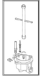
Unscrew the injector and replace it with the stipulated injector for the new gas supply (see table below).
