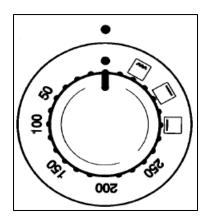
If you turn the secondary oven function selector and thermostat control knob clockwise, it will automatically select the conventional oven function and you can regulate the temperature between 50 - 250°C.
