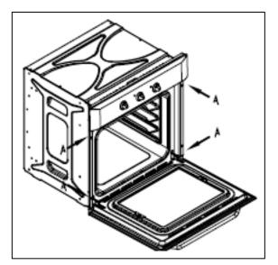
For both types of installation, ensure that the oven has been securely fixed into the housing unit. The fixing of the oven into the housing is made by using four screws (A). These should be screwed through the oven cabinet and into the housing unit.
