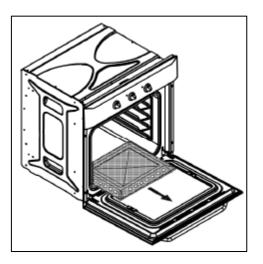
Open the door of the oven. Unscrew the fixing screws and then remove the base of the oven cavity (as shown opposite).
