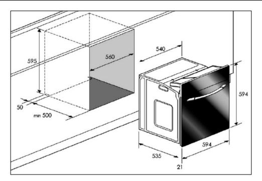
(**IMPORTANT:** The above drawing does not show the ventilation requirements that are necessary for installing this appliance, please refer to the installation instructions for this information).
