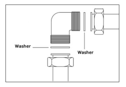
• A <sup>1</sup>/<sub>2</sub>" BSP female to female gas elbow should be connected to the gas inlet at the rear of the appliance and pointing in a downward direction. As indicated in the diagram above.
