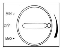
You switch on your appliance by connecting it to your mains supply and setting the thermostat. The thermostat control knob is located on the upper right hand side of the outside of the cabinet.
