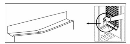
Defrosting occurs automatically in the refrigerator section during operation. The defrost water is collected by the evaporating tray and evaporates automatically.
