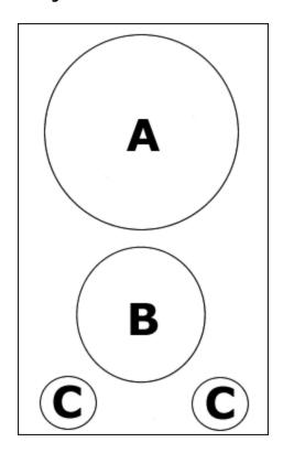
A =  $1.80 \text{ kW hyper-speed zone } (\emptyset 200 \text{ mm})$
