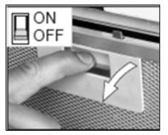
First lift up the cover screen and then remove the grease filters by pulling down on the handle and pulling them away from the cooker hood as shown in the diagram above.
