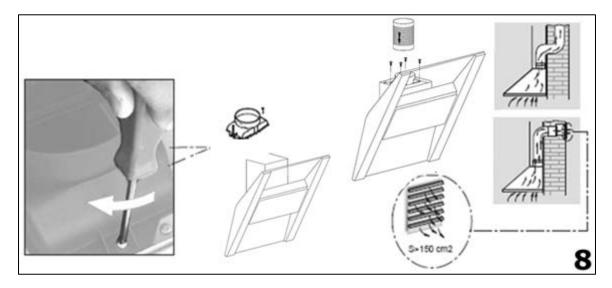
**8)** Connect the coupling to the top of the cooker hood, and then connect a 125 mm ducting hose to the coupling (please note that the ducting hose is not supplied with the appliance).
