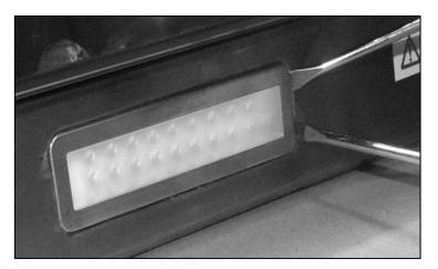
Once the light unit has been released from the fixture, gently pull out the light unit.
