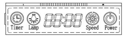
When you initially connect the cooker hood to the electricity supply, the backlight will turn on and the hood will enter standby mode. If no buttons are pressed the backlight will turn off again after 30 seconds.
