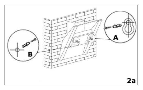
**2a)** The support screw holes are indicated by figure **A** in this drawing and the anchoring screw holes are indicated by figure **B**.
