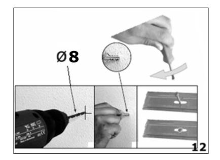
**12)** Using an 8 mm drill bit, drill out two holes on the pencil markings that you made in step 11. Insert rawl plugs into the holes and then use a screwdriver to secure the fixing bracket to the wall.
