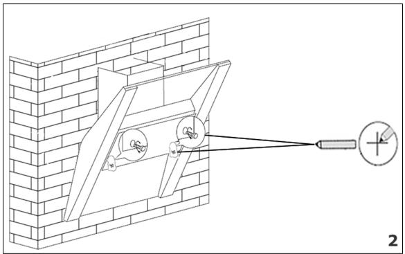
**2)** Position the hood against the wall that you are intending to install it on and mark the position of the screw holes that are to be drilled (as shown in the figure above).
