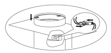
o Carefully locate the glass canopy over the main body of the hood.
