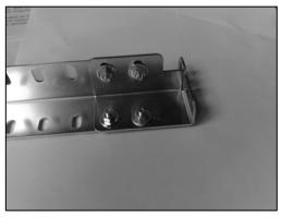
o Fix a connector piece to the bottom of each angle bar using the 10 mm x M4 nuts and bolts with metal washers (12 pcs).
