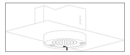
o Remove the fixing screw that holds the grease filter in place and then pull away the grease filter from the cooker hood.
