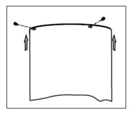
**7)** Slide the upper chimney section upwards and then use the self tapping screws (3 pcs) to secure it to the hanging plate.
