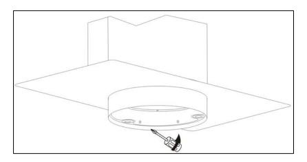
o Use a screwdriver to retighten the 6 fixing screws that hold the light board in place.
