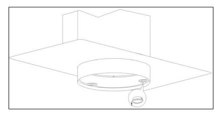
o Push the light back into the exposed hole in the hood and reconnect the light wiring point (see page 21 for a line drawing that shows how to reconnect the light wiring point).
