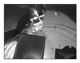
**4)** Locate the holes on the top of the main body of the cooker hood that you fix the connector pieces and angle bars to.
