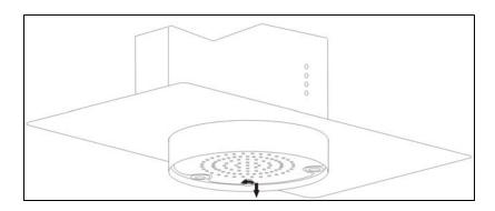
Remove the fixing screw that holds the grease filter in place and then pull away the grease filter from the cooker hood.
