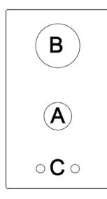
**A** = 1.00 kW auxiliary burner
