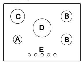
**A** = 1.00 kW auxiliary burner
