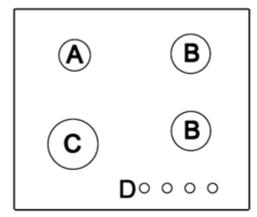
**A** = 1.00 kW auxiliary burner
