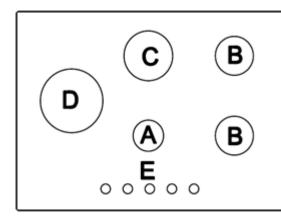
A = 1.00 kW auxiliary burner
