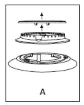
o Remove the pan-stands, burners and flame spreaders (A).
