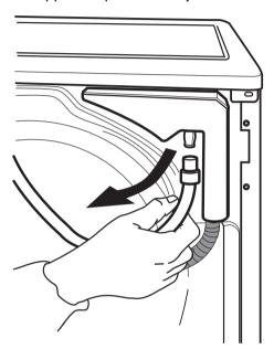
**B.** Remove the white hose from the hose fixation.
