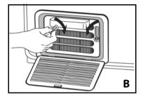
**c.** Hold the heat exchanger as shown in the picture. Clean it under running water by turning it around to reach all sides, especially in front and behind. Wipe away dust and lint from the heat exchanger seals and plates.
