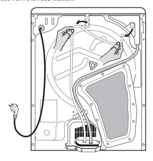
**C.** Fix the hose to the sewage system. The height difference between the floor where the dryer stands on and the connection at the sewage system should not exceed 1 m.
