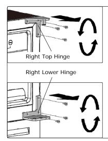
o Remove the right top hinge and right lower hinge.
