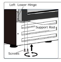
Install the door to the left hinge side by tightening the Support Rod with the 2 screws.
