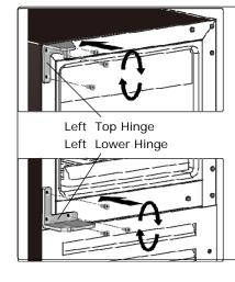
Take the left top hinge and left lower hinge from the plastic bag that contained this manual then install them in the designated positions on the left side of the cabinet.
