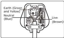
As the colours of the wires in the appliance's mains lead may not correspond with the coloured markings identifying the terminals in your spur box, please proceed as follows:
