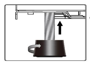
o Twist the foot into a suitable position to level the cabinet.
