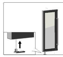
o Insert the Support Rod into the Left Lower Hinge hole of the door
