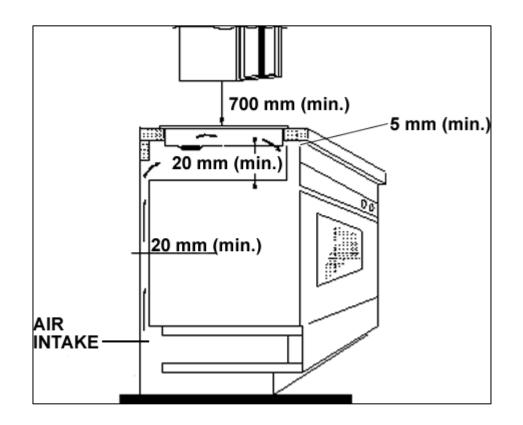
• **IMPORTANT:** You must observe the ventilation requirements shown in the drawing above. In particular the 20 mm gap underneath the hob and the 5 mm gap underneath the front edge of the worktop.
