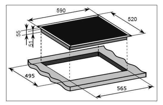
• Cut a hole in the worktop that corresponds with the drawing shown above.
