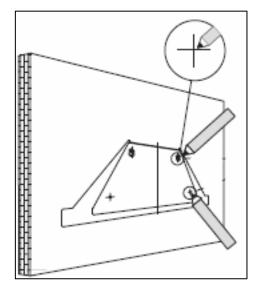
**2)** Position the hood against the wall that you are intending to install it on and mark the position of the support holes that are to be drilled (as shown in the figure below).
