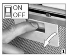
1) Remove the grease filters.
