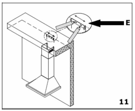
**11)** Take the fixing bracket (**E**) and place it between the two pencil marks that you made in step 9
