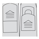
Slide vent cover on hose grip open to reduce suction if required.
