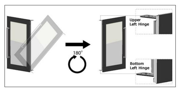
4) Screw the 8 screws of the upper left hinge and bottom left hinge tightly to fix the door in place.
