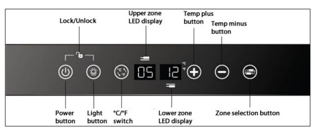
The control panel is located in the middle of the appliance.
