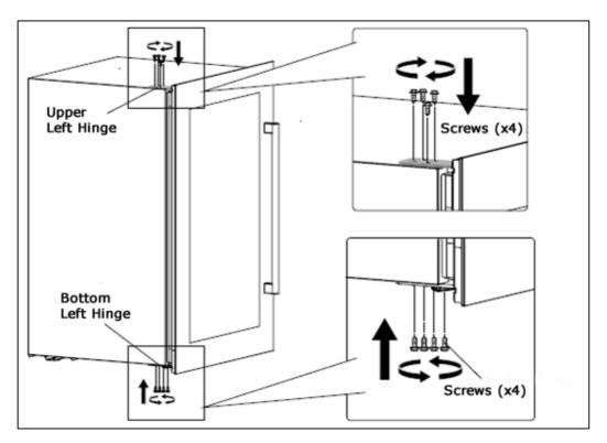
**IMPORTANT:** Check that the door opens and shuts correctly, without fouling, after you have completed the door reversal process.
