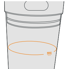
Don't over fill the dirt container to avoid clogging your filter
