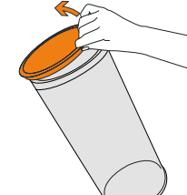
Tap the filter over a bin to remove the dirt
